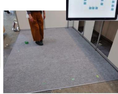
"floor sensor" is a device that can detect human movement without any obtrusive equipment, as the sensor can be hidden under the floor. This technology has versatile applications, including monitoring the elderly for safety and security purposes.
