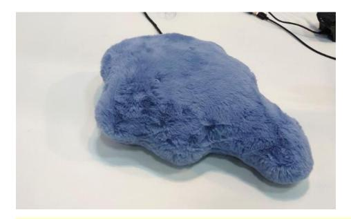
A "stuffed animal robot" that can identify touches on various parts of its body, allowing for diverse interactions with the robot (such as petting its head or hugging it) and changing its responses accordingly.
